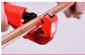
1. Cut the tube to length
