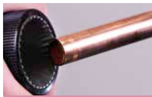
2. Deburr and remove all external sharp edges
