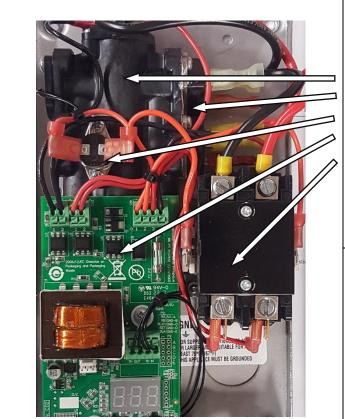
Heating chamber Triacs Energy cut-off (ECO) Control board Contactor
