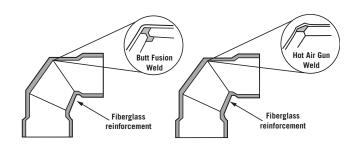
Butt Fusion Fabricated Fitting
