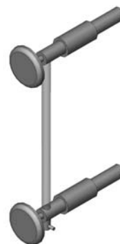
Figure 6.4: Gauge Glass Installation
