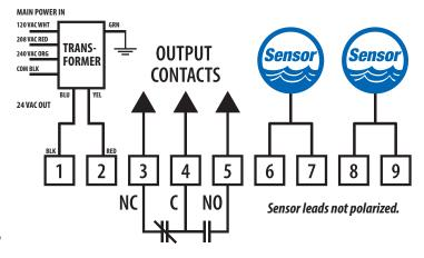
5. Turn off the main power. Wire the appropriate inputs to the main power source. Wire the blue and yellow wires (24 VAC output) to the plenum wire that is prewired to the power input of the contact plug. Turn on the main power. The green Power indicator light on the receiver will turn on.
